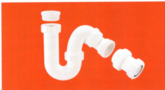
Tubular HandiTrap 75mm water seal with 1 1/4" and 1 1/2" inlets and outlets. Note: Trap outlet can be swivelled from 'P' to 'S' position
